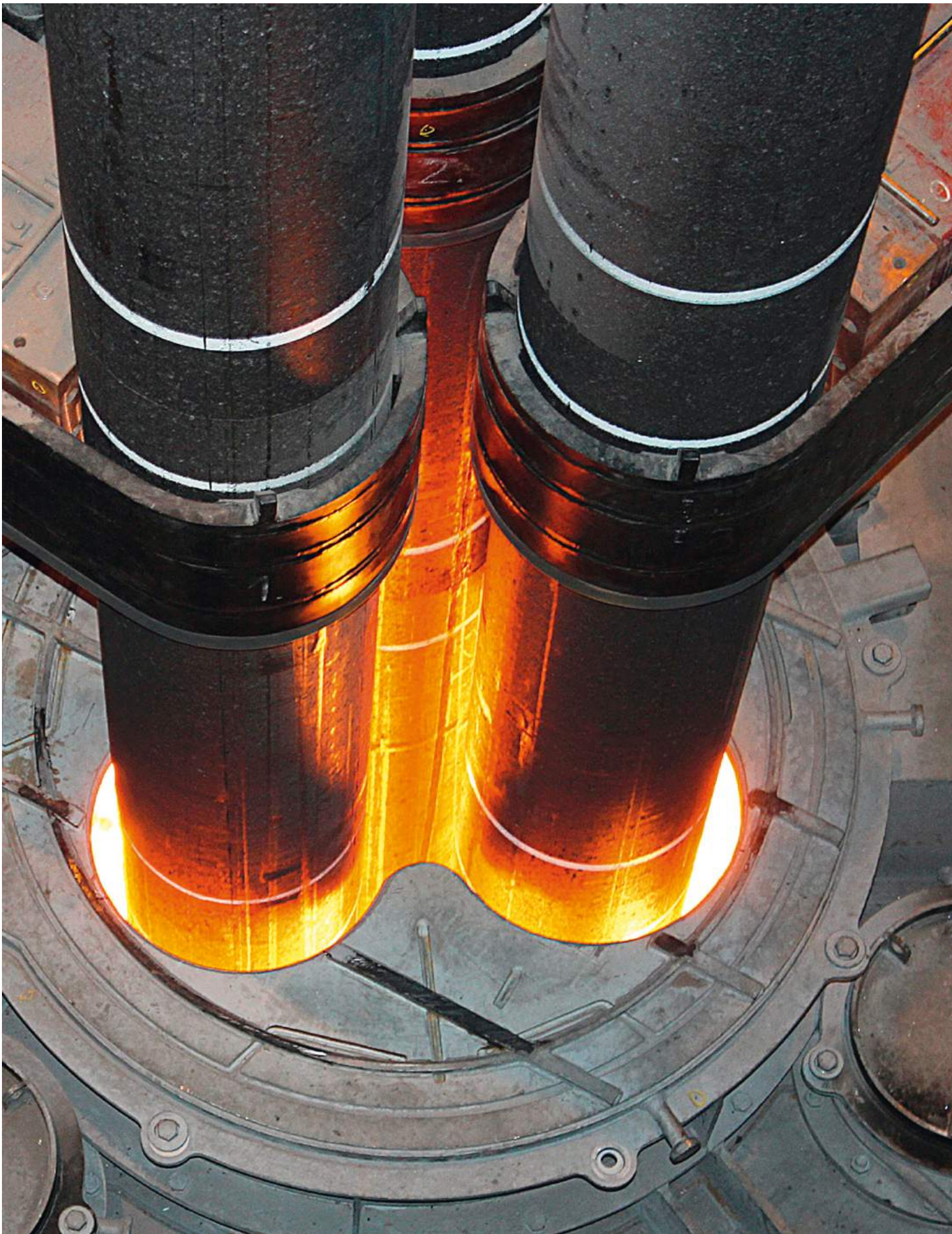
LD steelmaking plant Völklingen, secondary metallurgy: Ladle furnace
