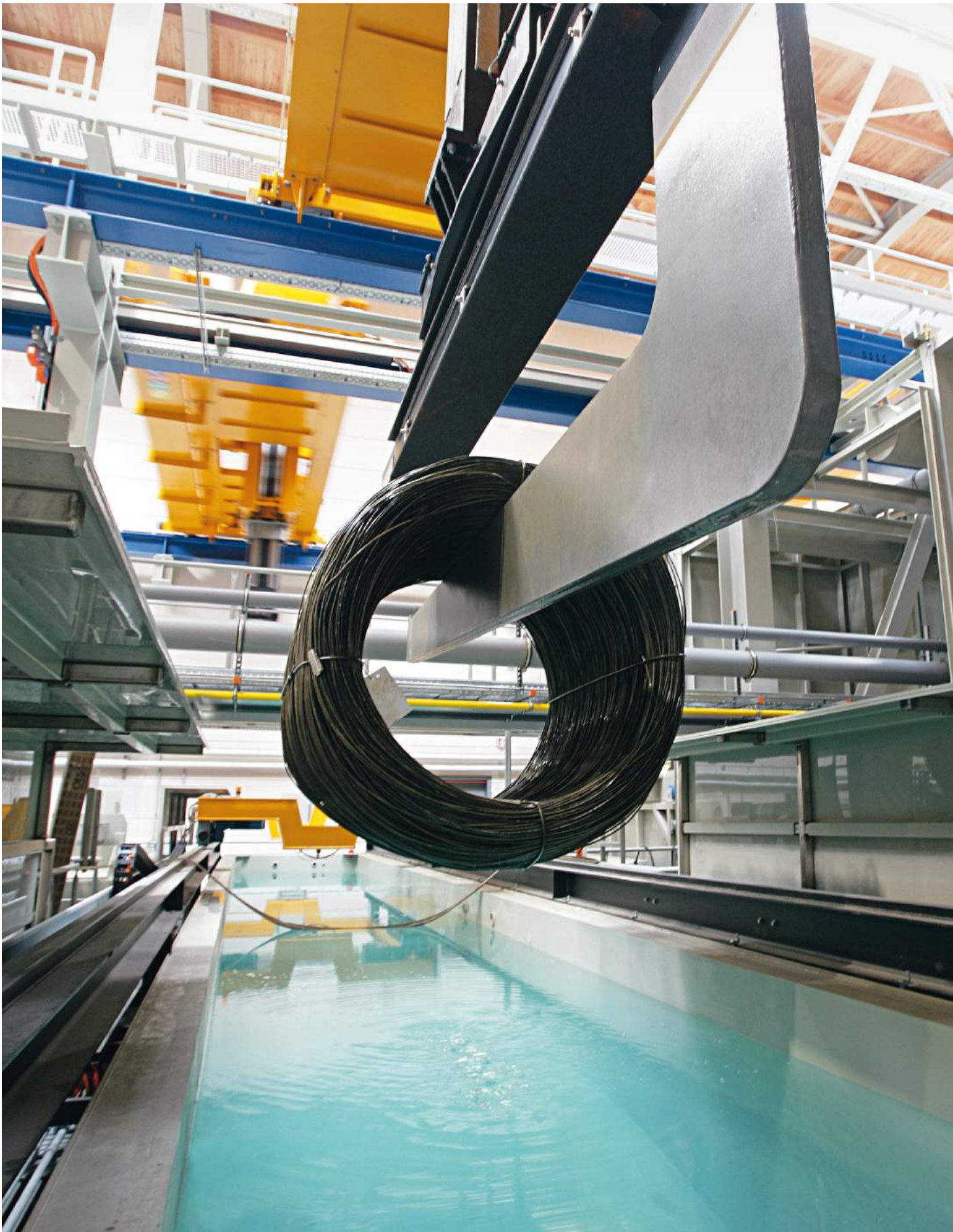
Drahtwerk St. Ingbert: New pickling line
