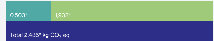
Heavy plate (Dillingen, Dunkerque) via BF/BOF
